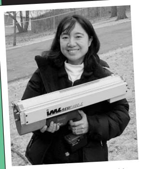
This machine helps Kyoko decide if a tree is hollow and should be cut down.
